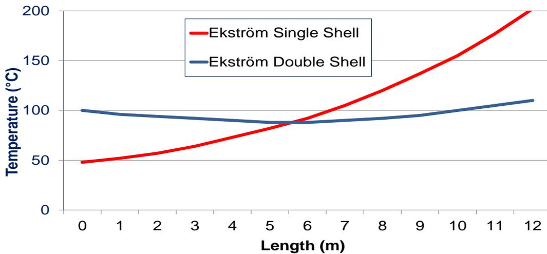
Figure 2: Temperature difference between tube and carbon black gas at 800°C
