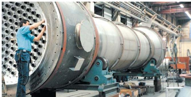
**Figure 1: Assembly of air preheater in the Ekstrom workshop, south Sweden**
