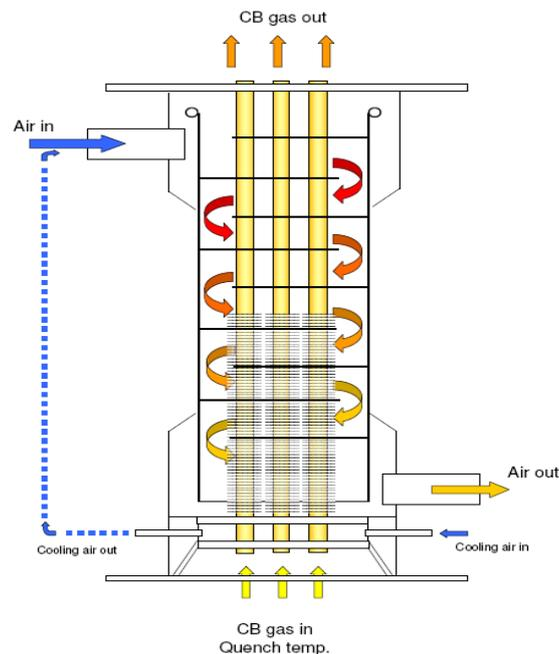
Figure 2: Ekström Single Shell 900°C Carbon Black Air Preheater
